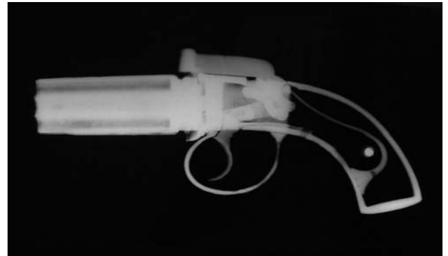
Fig. 4: Radiograph of pistol showing internal components.
